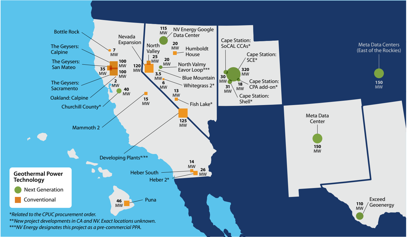
Figure 16. New geothermal power project developments within PPAs signed between 2021 and July 2025, including those related to the 2021 CPUC procurement order. Data from multiple sources; see Table 3 for more information. Note that CCA stands for Community Choice Aggregator, SCE stands for Southern California Edison, and CPA stands for Clean Power Alliance.
